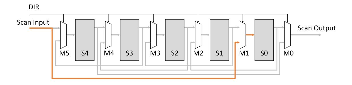
Right to Left (R2L) shift operation - DIR pin is de-asserted (DIR = 0)
